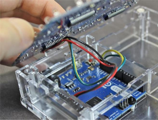
Now the Trellis gets turned over, LED side up, and is lowered into place in the case. You'll see the horizontal and vertical braces have notches into which the board neatly fits.
