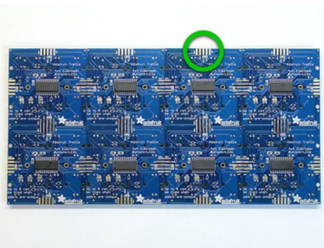
On the HELLA UNTZtrument — a 4x2 assembly of Trellises — connect the wires to the third header along the top edge, not the rightmost fourth header.
