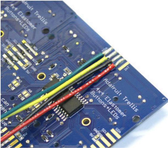
Try pointing the wires “inward” rather than off the edge of the board. This makes it easier to fit in the case.
