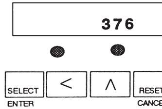
After one of these options is displayed for a second, the value for this option is automatically displayed. Once the option value is displayed, pressing the < key will move one digit to the left and the ^ key will increment the value by one. Then the SELECT key must be pressed to save the new value. Pressing RESET will return to the Process Count display. If SELECT is not pressed after a change, RESET will return to the count display and the change will not be entered.
