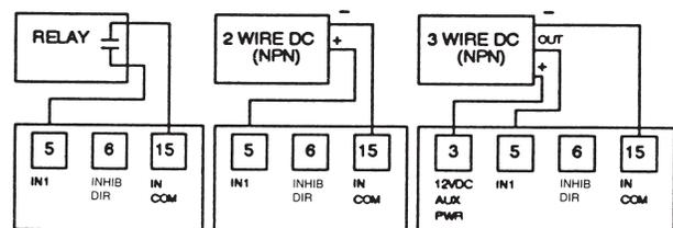
**COUNT INPUT WIRING - SOURCE INPUT SIGNAL**
