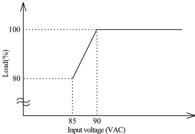
The following input voltage derating curve assumes maximum output power is 100%
