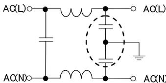
The example of noise filter circuit that may increase capacitance value between “Input and  $\perp$ ”
