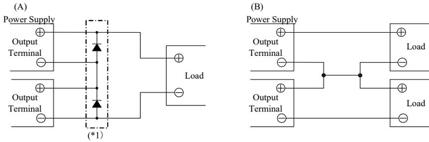
(\*1) In case of (A), please connect bypass diodes to prevent reverse voltage. Please select a bypass diode with maximum forward current rating more than output load current. And maximum reverse voltage must withstand each power supply output voltage.
