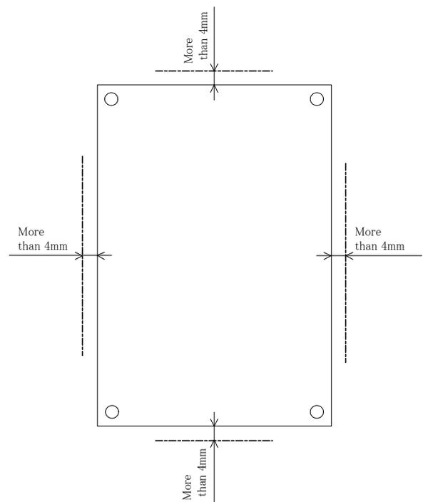
Keep 4mm space from the surfaces and sides of PCB. Especially, 8mm space is necessary from the solder surface.
