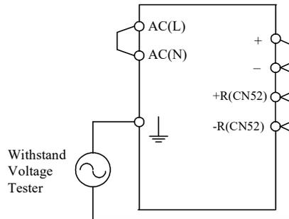
Note 1 : This product have monolithic ceramic capacitor in secondary circuit to  $\perp$ .
