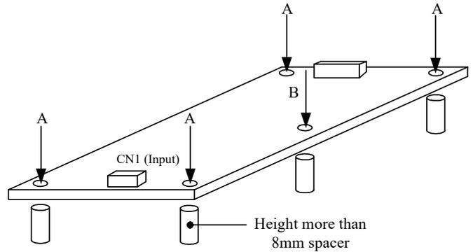
Allowable area by metal pieces is 9mm from each PCB corners. Refer to figure below.
