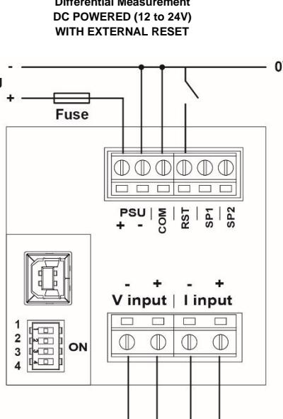
Note: When using a DC PSU, always link PSU negative to COM terminal
