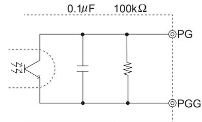
Fig.1.6 Internal circuit of PG
