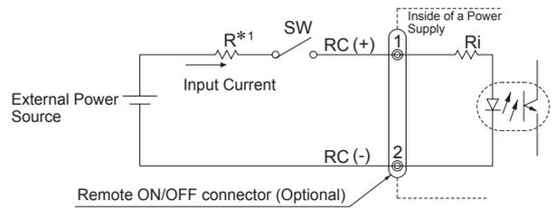
Fig.7.7 Example of using a remote ON/OFF circuit
