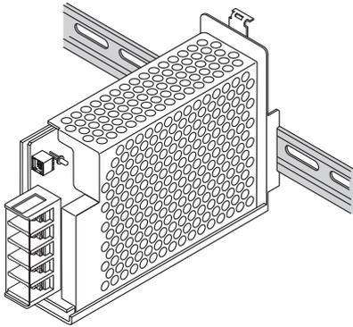
Fig.7.8 Power supply installed on a DIN rail
