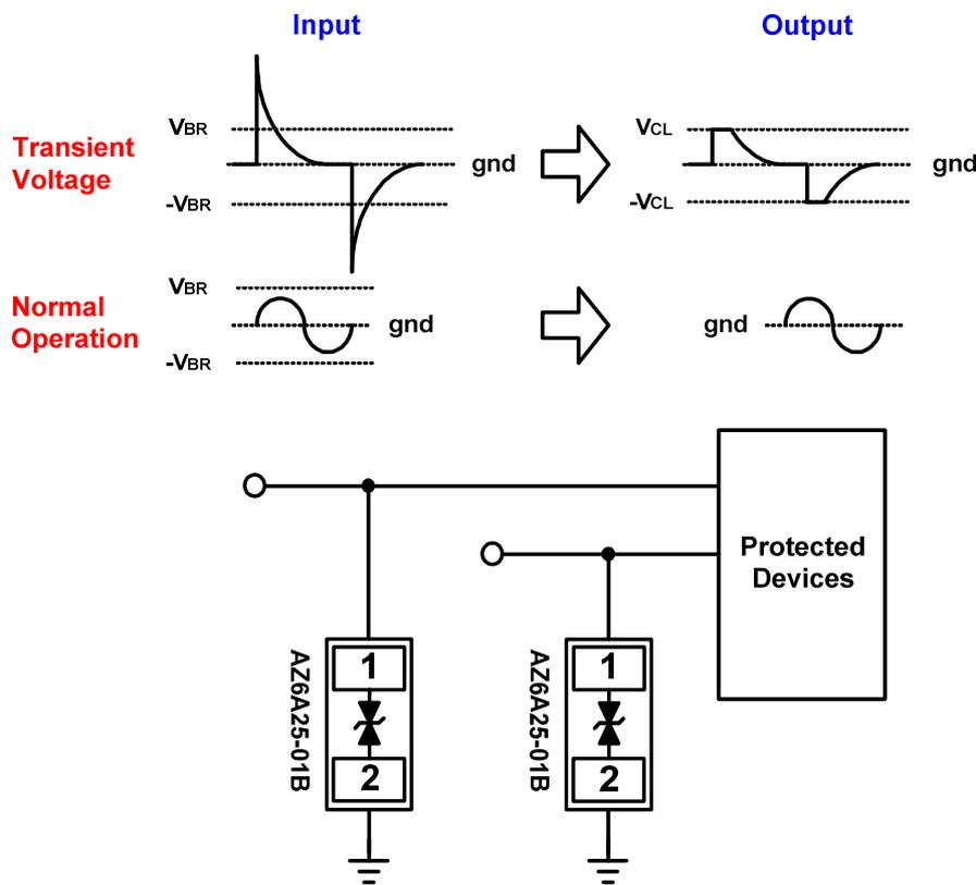
Fig. 1 ESD protection scheme by using AZ6A25-01B.
